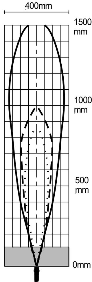
Beside the three typical cone shapes for the DUPR-A sensors are shown (small, medium and large cone). Furthermore, the size of the detection beam is influenced by air temperature and humidity. The colder and dryer the air, the larger is the beam.
